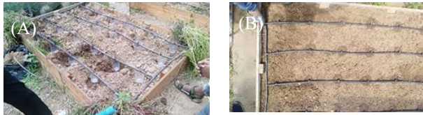
Figure 4. Emitter flow rate measurement in the box of soil.
