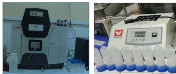
Fig. 2. AAS machine used for Fe, Mn, and As analyses
